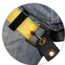
Tongue buckle and grommet fasteners are corrosion resistant to ensure smooth, consistent operation. Grommets are inserted through an opening in the web as opposed to a punched hole to maintain webbing integrity. Consistent spacing ensures a custom fit regardless of user size. Harness sizing adjustment is easy, especially when wearing gloves.
